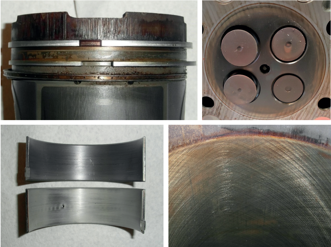
Engine parts after 5793 running hours on SENTRON SP 30
